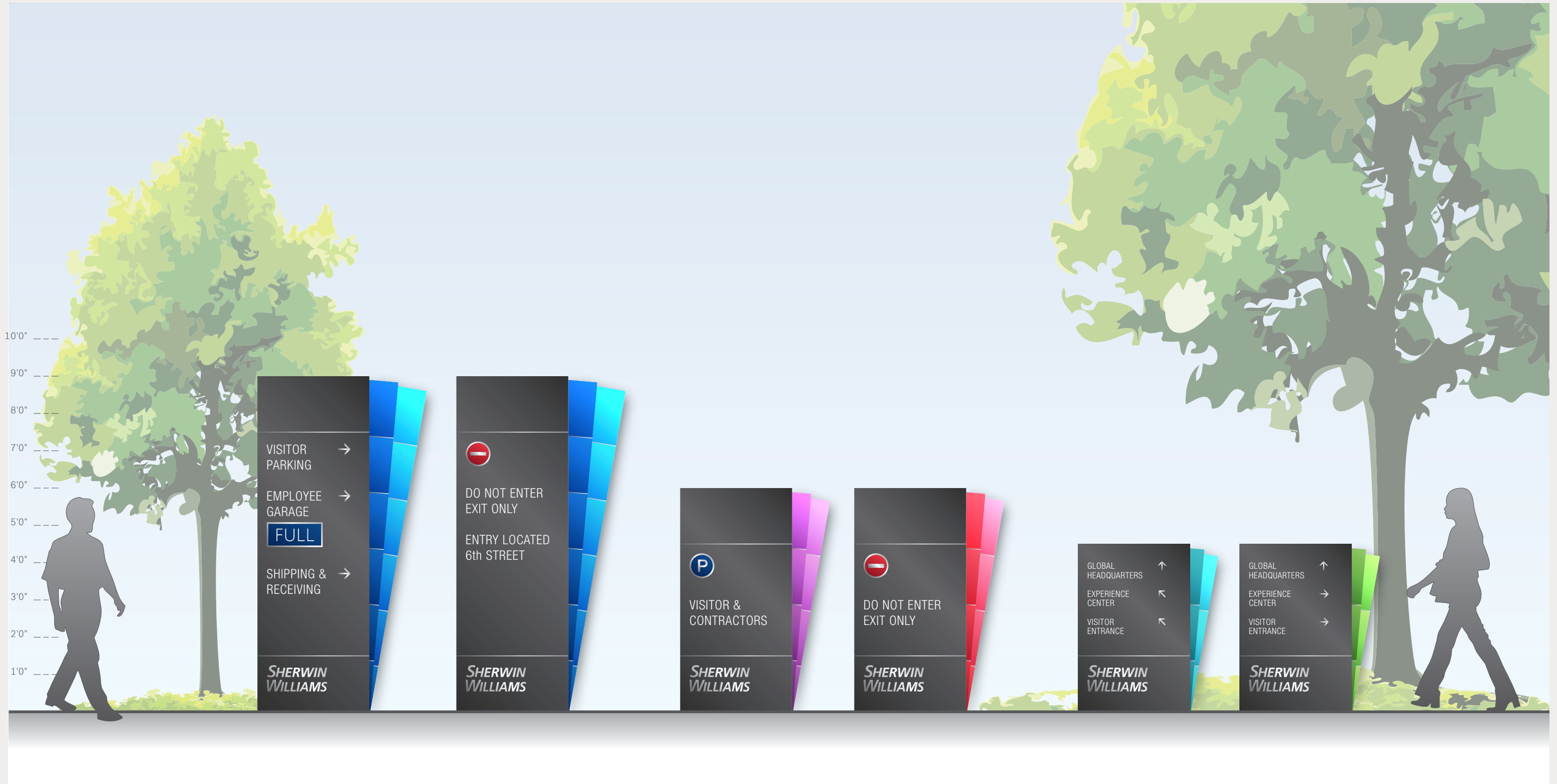
ELEVATION: VEHICULAR & PEDESTRIAN DIRECTIONALS – FRONT SCALE: 3/8" = 1'0"
